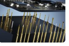
For the in-circuit and functional test of PCBs basic probes in the centers 50 mil, 75 mil and 100 mil are most commonly used. In these applications long lifetime, reliable contacts and great variety of tip styles and spring forces are essential. FEINMETALL offers the compatible receptacles for all its basic probes. All common connection types are supplied (e.g. WW, solder, crimp, wireless).
